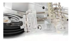
The RC10CC suspension gives you all the adjustability of full-size race buggies. The A-arm/Ball joint design allows precise camber, caster, ride height, and spring rate tuning. The adjustable VariLok differential is included, and the updated chassis fits 6-cell NiMH and 2S LiPo battery packs.
