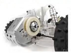
Independent suspension with coil-over shocks help smooth out the bumps. Precision-molded, nylon suspension components can be easily custom color dyed. A-Arm/Ball joint design permits static camber, camber rise, caster, ride height, and spring rate tuning to suit every type of track.
